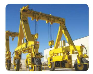
Structure with an articulated union Automatic steering alignment Hydraulic stainless steel piping Cooled Diesel propellent motors
